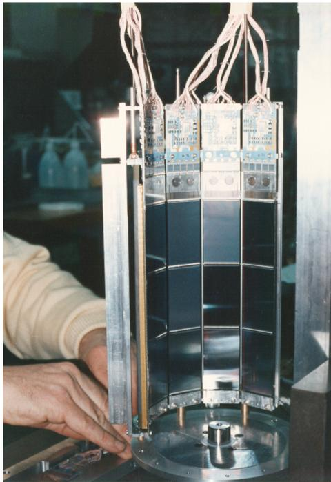
Figure 9: Part of the OPAL Si vertex detector.
