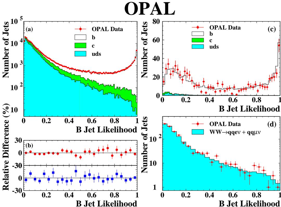
Figure 10: An example of the b-tag performance/modeling checks. (a) and (b) show the comparison between data and MC simulations. (c) B-tagging over the  $b\bar{b}$  sample taken at the  $Z^0$  peak. (d) The semi-leptonic WW sample that should contain no b jet.
